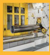
The new RFFM Series now brings about multi rollers for the production of dimensionally precise, tubular hollow work pieces. The fixed roller housing of the CNC controlled machine can be equipped with three, four, five or six rollers depending upon customer requirements, including extremely large diameter part productions!
